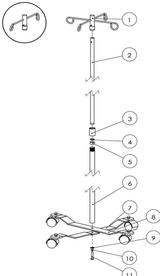
The diagram illustrates the assembly of an I.V. stand. It shows a vertical pole with a hook at the top and a base at the bottom. The parts are numbered 1 through 11. Part 1 is a hook, 2 is a cannulation, 3 is a knob, 4 is a bushing A, 5 is a bushing B, 6 is another cannulation, 7 is base A, 8 is base B, 9 is a plain washer, 10 is a single coil lock washer, and 11 is a bolt. The assembly steps are detailed in the installation procedure.
